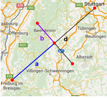
Figure 20: The structure of the rotated ellipse. Both cities are the endpoints of the major axis. d represents the distance between both cities. a is half of the distance and represents the length of the minor axis. b is half of a . Both variables a and b are then used to build the ellipse. This is how we imagined a nice ellipse, the variables can easily be changed to create different ellipse structures.
