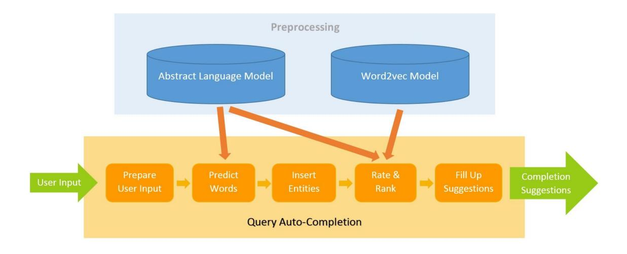
Basic pipeline of the Auto-Completion algorithm.
