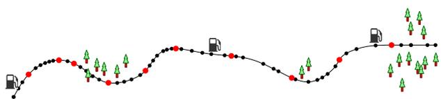
**Fig. 2** Route with nearby gas stations and forest areas. Red nodes indicate a subsampling resulting from a global cover computation. Querying only the red points instead of all points to identify gas stations or path sections through the forest is much faster, but still sufficiently accurate
