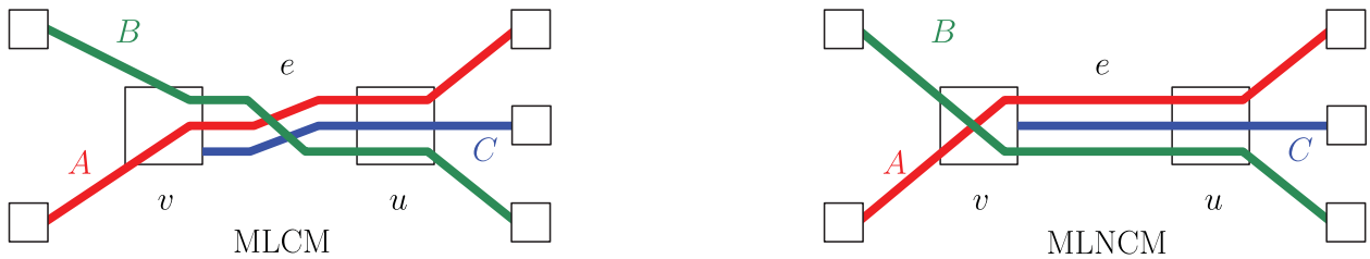
Figure 11. A line graph G with line orderings in the MLCM formulation (left) and our MLNCM formulation (right). Under MLCM, crossings are not allowed to occur in nodes and must happen on edge e . Under MLNCM, crossings are only allowed at nodes.
