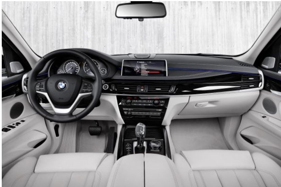
Figure 4.4: Cockpit of car prototype. The basis for this prototype is constituted by a BMW X5 xDrive40e. The display in the center is being used for the notifications and warnings given by the V2X-application. Image source: [46].
