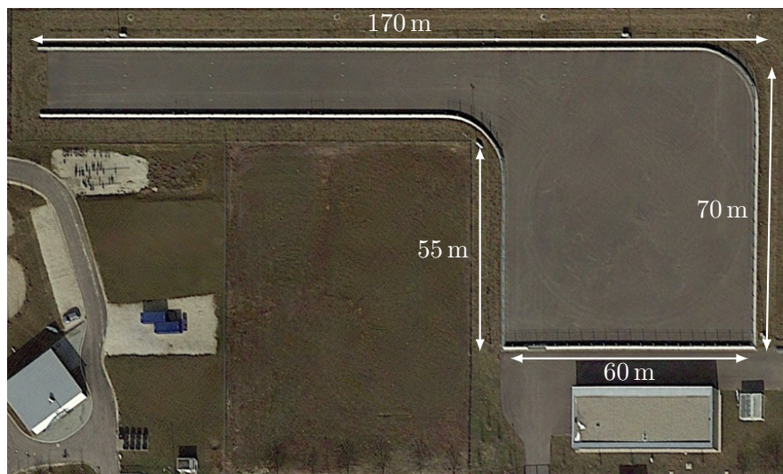
Figure 5.18: Aerial view and dimensions of CARISSMA Test Track in Ingolstadt. Image source: [58]
