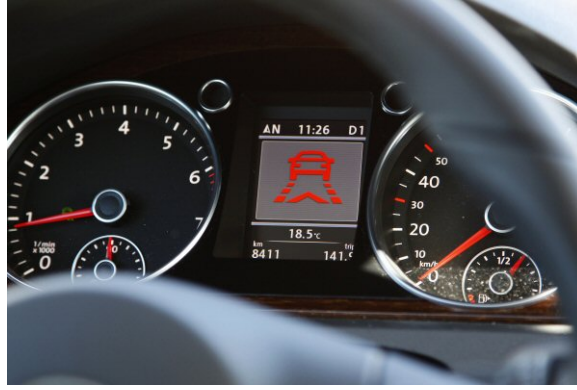
Figure 2.5: Example of a warning given by a HMI. The shown HMI corresponds to a Forward Collision Warning on a VW Passat. This sensor-based solution measures the distance to the vehicle ahead and uses the difference of speeds for estimating if a collision is probable. If it is, a visual warning, usually accompanied by auditive and/or haptic signals, is given. Image source: [38].
