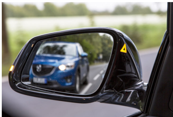
Figure 2.4: Example of a notification given by a HMI. The shown HMI corresponds to a Blind-Spot Monitor on a BMW Hybrid Active 3. This is a sensor-based solution which detects the presence of vehicles located in its blind-spot. When an intention of changing lanes is detected by the system, a yellow triangle is illuminated for making the end-user aware of the other vehicle. Image source: [37].
