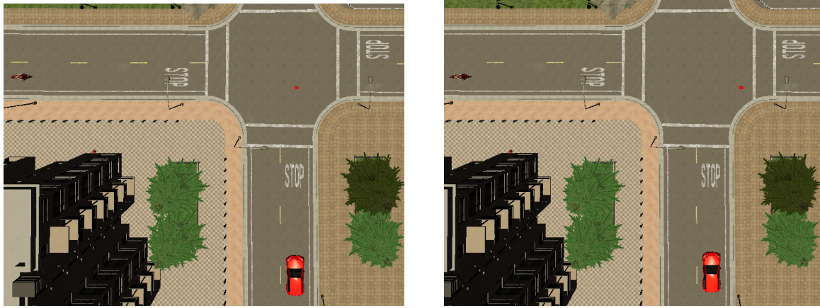
Figure 4.13: Point-of-Collision estimation based on the use of map data. The Point-of-Collision estimated using map data is represented by the red dot inside of the intersection. In the left picture, both vehicles intend to drive straight across the intersection while, in the picture on the right, the car is intending to perform a right turn.
