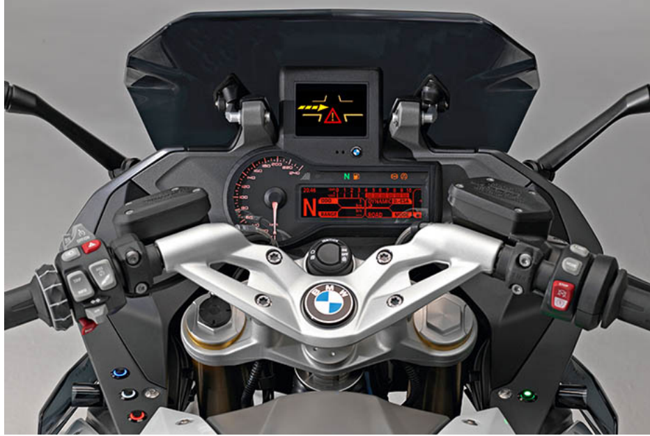
Figure 4.3: Cockpit of motorcycle prototype. The basis for this prototype is a BMW R 1200 RS. Located above the instrumental panel is an additional display for the notifications and warnings given by the V2X-application. Image source: [45].
