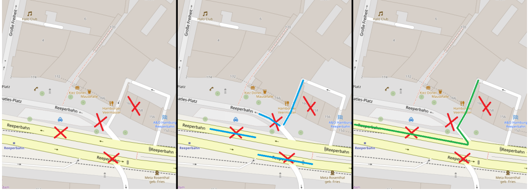
Figure 2: This figure illustrates map matching. The left image shows GPS points with a natural inaccuracy. The image in the middle illustrates that a simple metric like always choosing the closest street is not a valid option when it comes to map matching. The image on the right shows a desirable map matching for the given coordinates.
