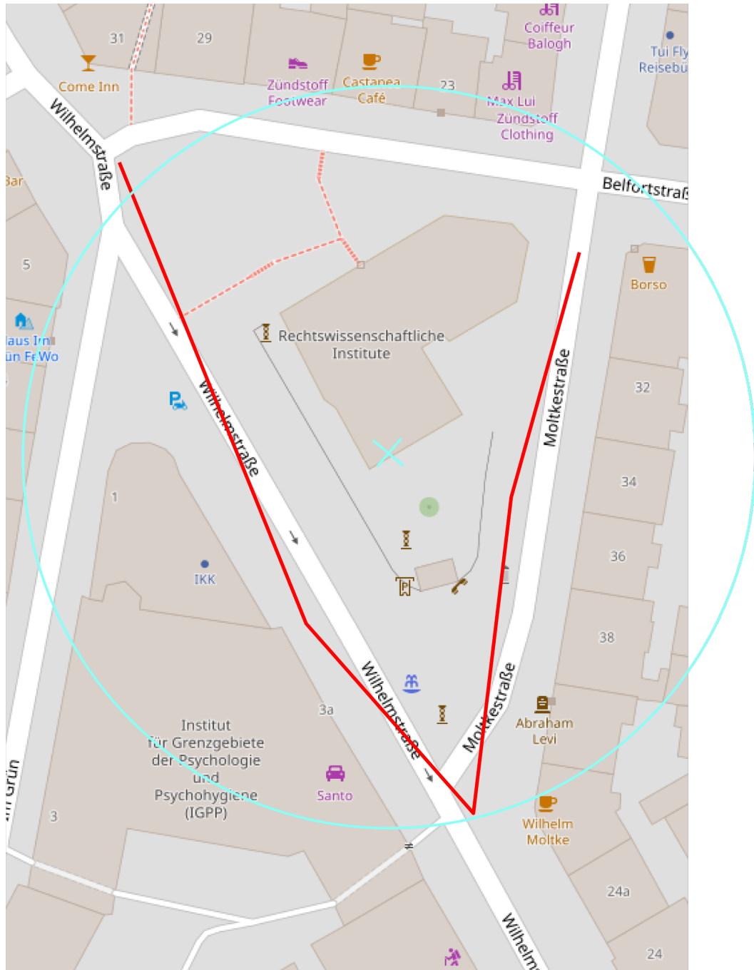
Figure 18: are_last_gps_points_close_to_each_other is not perfect: Let us assume that there is a shape with a bus drives along the painted GPS point sequence. In this case, the function would remove the GPS point in the upper right corner from L to soften the impact of outliers. Then, none of the remaining points in L would be further away than the radius allows and the function would return True . Cases where a shape follows an acute angle are therefore susceptible to failures.
