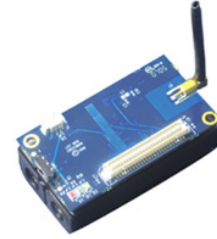
Figure 2. IRIS Mote: An IRIS mote used in our experimental evaluation. The mote has 128 KB of flash, 8 KB of RAM, and it uses an 8-bit AtMega128L processor. It is powered by two AA batteries and is equipped with a 2.4 GHz radio for communication with other motes.
